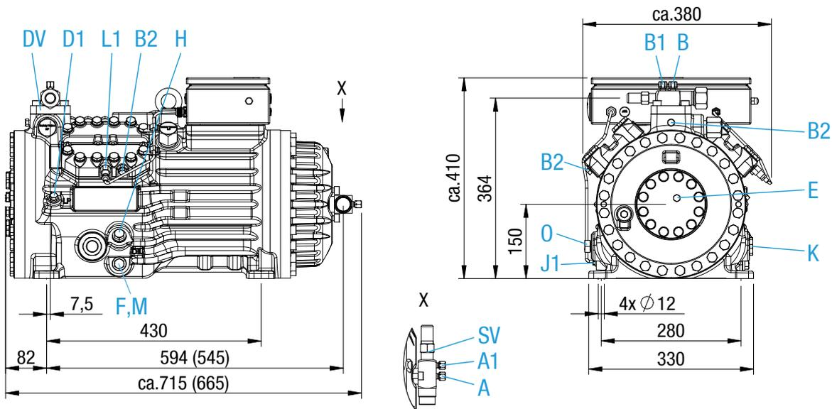
Dimensions in ( ) = HGX34/110-4 CO<sub>2</sub> T    HGX34/130-4 CO<sub>2</sub> T    HGX34/150-4 CO<sub>2</sub> T    HGX34/170-4 CO<sub>2</sub> T    HGX34/210-4 CO<sub>2</sub> T
