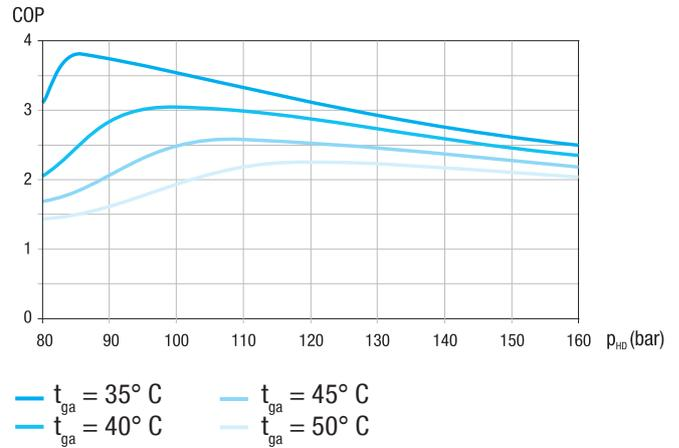
$t_{ga}$  = Gas cooler outlet temperature
